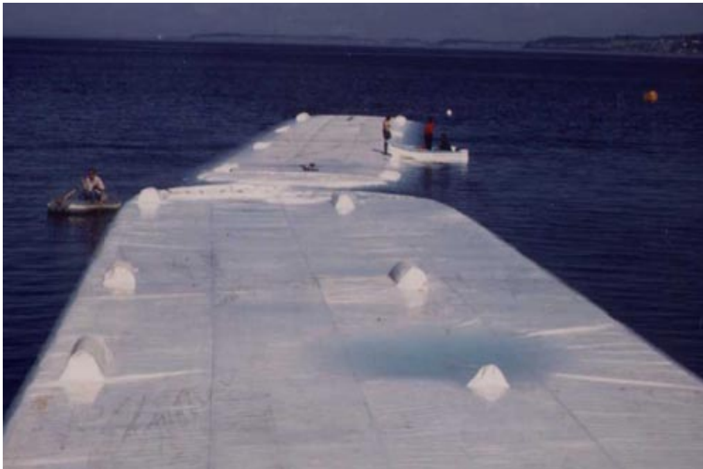
Two connected Spragg Bags™ during demonstration voyage in Washington State, USA. The waterbag in the foreground is being filled and the waterbag in the background has been filled.
